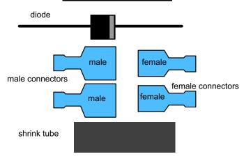
**STEP 1:** Trim each lead on the diode to 3/8" long, as shown.
